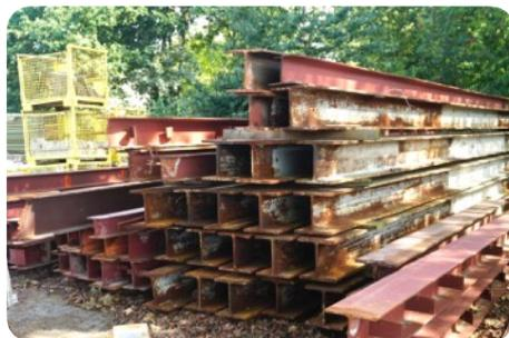
Storage of reclaimed steel beams, coated with corrosion protection (in red) and uncoated (rust and white paint) © [Gebruikte bouwmaterialen Weert](#)
